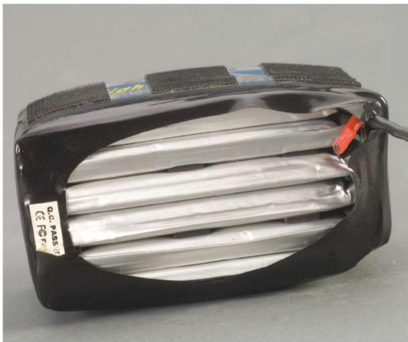
This an example of a battery that is either being run too long each flight, or being pushed harder than its rated for. A puffed battery like this is at the end of its life cycle and is ready for disposal.
