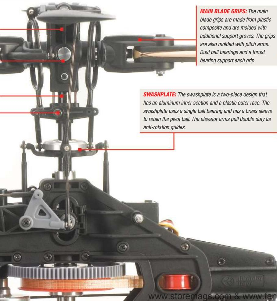
**MAIN BLADE GRIPS:** The main blade grips are made from plastic composite and are molded with additional support grooves. The grips are also molded with pitch arms. Dual ball bearings and a thrust bearing support each grip.
