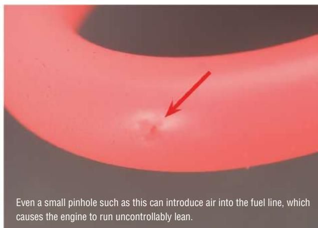
Even a small pinhole such as this can introduce air into the fuel line, which causes the engine to run uncontrollably lean.
