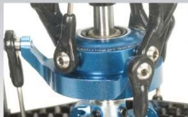
**SWASH CONTROL:** The swash is controlled by a 120° CCPM configuration with direct input linkages.
