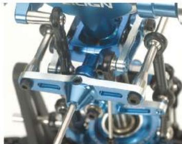
**BELL/HILLER ARMS:** The aluminum Bell/Hiller arms are mounted underneath the main blade grips to the flybar seesaw. The arms are dual ball bearing supported but do not offer any input or output options.
