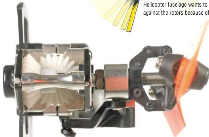
The pitch slider transmits control inputs that increase or decrease T/R pitch and thrust.
