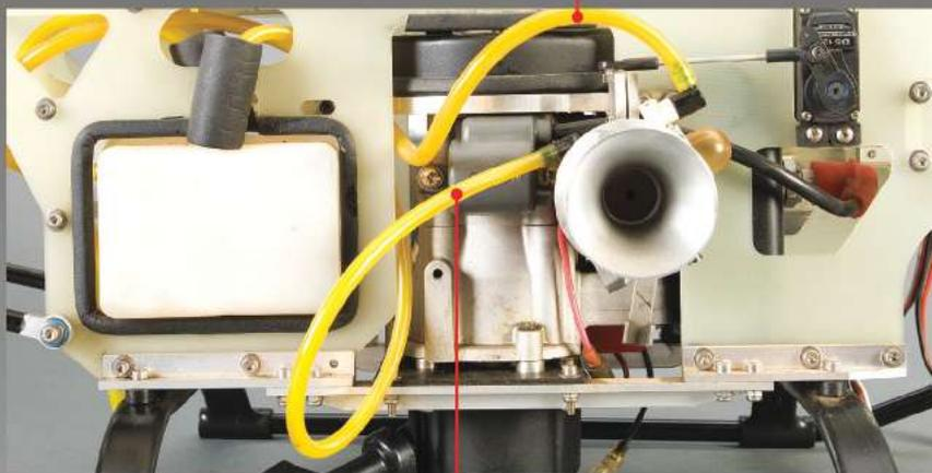
**RETURN LINE (ON SOME MODELS)** • Some fuel tanks will have a third tap built in, which is used as an excess fuel return line. On engines that use a fuel pump, there will often be an excess amount of fuel above what the engine needs to operate. This fuel is sent through a bypass line back to the fuel tank so that no fuel is wasted and a constant fuel pressure to the carb can be maintained. Fuel tanks with return taps will have the tap on the bottom of the tank.
