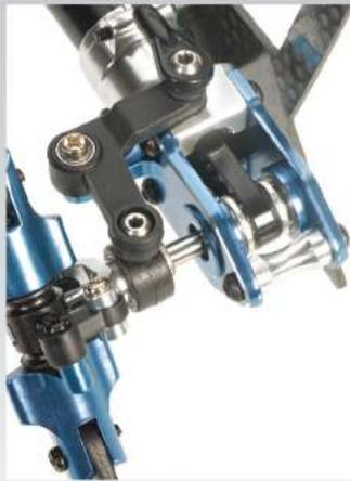
**TAIL CASE:** The tail case has been completely redesigned to better withstand crashes. The case is made completely from aluminum and beefed up to prevent bending. The tail case is comprised of three pieces: the boom clamp and two side plates. One side plate is machined with the pitch actuator standoff, making it stronger.
