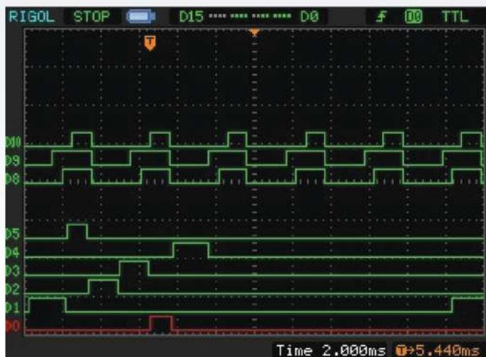
Overdrive inserts additional position pulses in between the actual received pulses.
