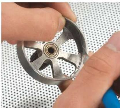
**2** Use a sharp hobby knife and carefully remove the old liner material from the clutch bell. Be careful and take your time during this process, it is very easy to slip and cut your fingers. A safer alternative is to use a rag around the pinion and lightly clamp on to the clutch bell using a vice.
