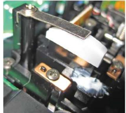
A plastic detent cover makes the collective smooth as glass. It can be relocated to the other gimbal should you decide to change the stick mode.
