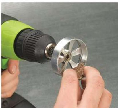
**3** After most of the material is removed, take some coarse sandpaper and sand the rest of the material off. If there is some residue left on the clutch bell, take a cotton swab soaked with acetone to remove the glue. At this point you can chuck the end of the pinion in a drill and give it a nice once over with the sandpaper and drill. This will create a rough enough surface for the new liner to adhere to.
