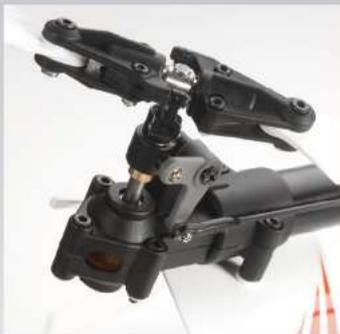
**TAIL CASE:** The tail case is a two-piece split design that has a guide pulley located just before the tail rotor drive pulley. The case is made from plastic and has all the parts needed for the pitch actuating system molded into the design. The tail case clamps on to the tail boom using two screws that also hold the vertical tail fin.
