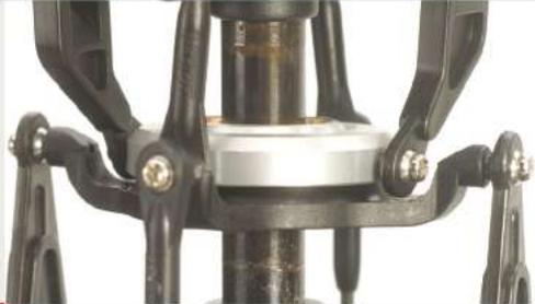
**DESIGN:** The frame is a composite plastic material that is molded to have every support, bearing block, fan shroud, and mounting point in one simple design. This design has made the Raptor what it is today. Fewer parts allow the Raptor to remain one of the most reliable airframes available.
