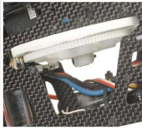
**AUTOROTATION DRIVE:** A one-way bearing is pressed into the main gear hub and links the main tail gear to the main rotor gear. This allows for the tail to be driven during an auto. The hub is secured to the main gear using four machine screws that thread into the main gear. No other bearings are used to support the autorotation drive.
